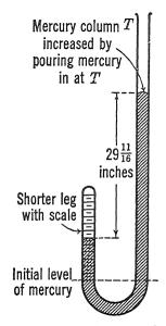
Fig. 13. Boyle's J tube, with a scale on the shorter leg reading 24 as compared to the initial reading of 48 (see Table 1, Column A).
