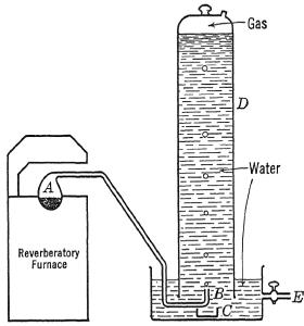
FIG. I. Diagram of apparatus used by Lavoisier in collecting the gas evolved when red oxide of mercury is heated.
