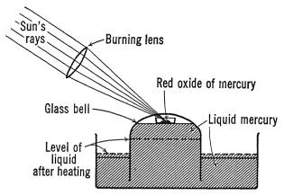
FIG. 2. Priestley's method of heating red oxide of mercury with a burning lens.
