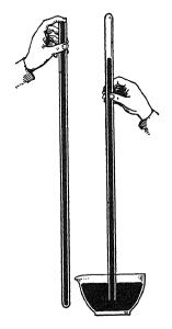
FIG. I. Torricelli's experiment with a column of mercury in a tube longer than 30 inches.
