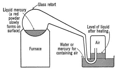
FIG. 3. Boiling mercury absorbs oxygen from the air.
