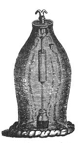
Fig. 11. The syringe of Fig. 10 mounted in a receiver and arranged to raise a liquid from a small vessel.
